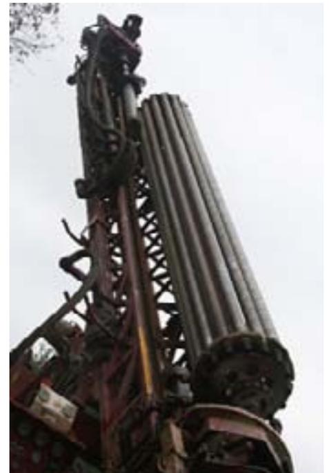
A 36-foot-tall drill was needed to install the geothermal system at the Gearon’s house in Derwood, Md.
